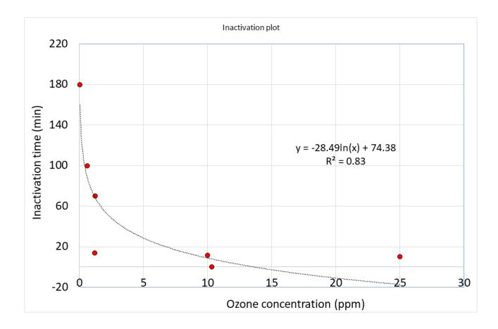
Fig. 1: relationship between ozone concentrations and contact time for viral inactivation.
