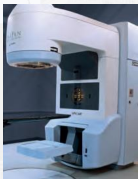
Amorphous Silicon Electronic Portal Imager Portal Vision As1000 (pixel size of 0.392 mm)
