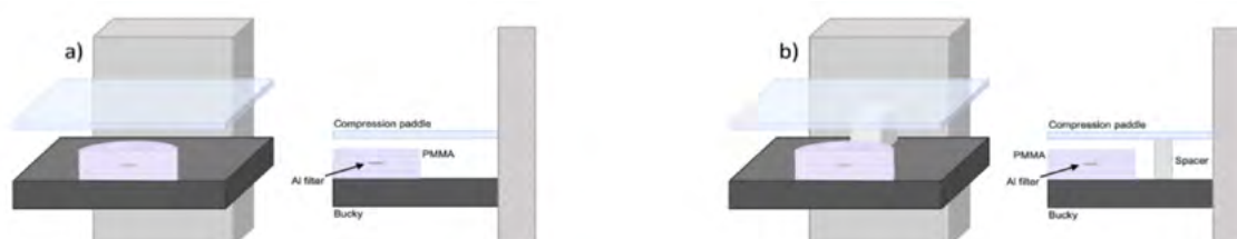
Figure. 3.2 Set up for the AEC performance test, front view and side view a) without and b) with spacer.
